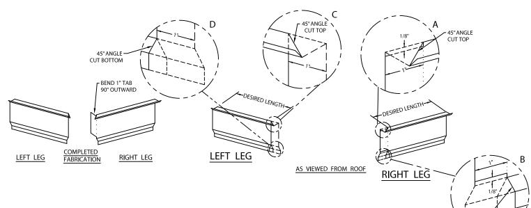
STEP 9 - INSIDE MITER RAIL FABRICATION (CUT RAIL TO DESIRED LENGTH)
