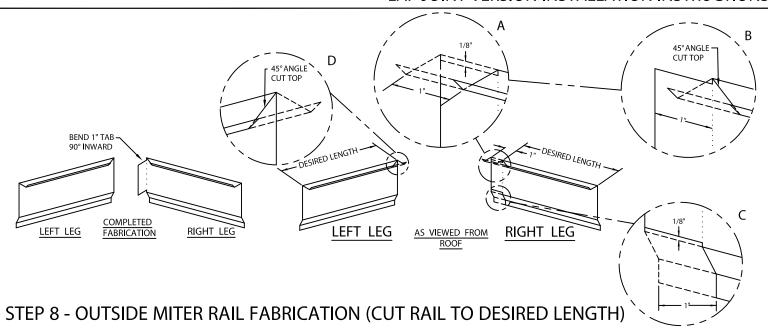
RIGHT LEG - DETAIL A: First remove a 1" section from top flange, 1/8" down face and 1" horizontally as shown to create tab. DETAIL B: Cut top flange at 45° angle. DETAIL C: Cut off bottom face at a 1/8" x 1" as shown and continue through area shown on bottom flange. Bend tab inwards 90°.
