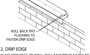
PLACE DRIP EDGE ON WALL. ROLL BACK TPO FLASHING TO EXPOSE FASTENING SLOTS AND FASTEN THRU PRE-SLOTTED HOLES 6" WITH PROVIDED NAILS.
