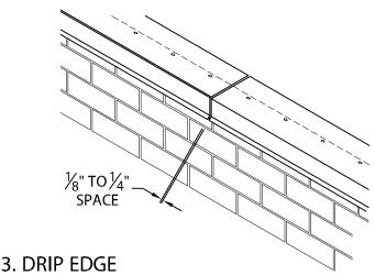
CONTINUE INSTALLING 12'-0" LENGTHS OF DRIP EDGE. LEAVE A  $\frac{1}{8}$ " TO  $\frac{1}{4}$ " SPACE BETWEEN PIECES.
