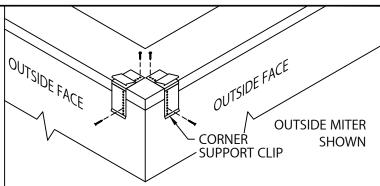
STEP 1 - CORNER SUPPORT CLIPS LOCATE AND FASTEN GALVANIZED CORNER SUPPORT CLIPS TO THE WALL.
