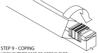
HOOK OUTSIDE FACE OF COPING OVER THE ANCHOR CLIPS AND ROTATE INTO PLACE. PRESS DOWNWARD ON REAR LEG UNTIL IT ENGAGES ONTO ANCHOR CLIPS.
