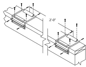
STEP 7 - ANCHOR CLIPS LOCATE AND FASTEN GALVANIZED ANCHOR CLIPS TO WALL AT 2'-0" CENTERS WITH PROVIDED FASTENERS FOR SUBSTRATE (SEE DETAIL A).
