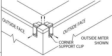
STEP 1 - CORNER SUPPORT CLIPS LOCATE AND FASTEN GALVANIZED CORNER CLIPS TO TO THE WALL.
