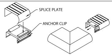
STEP 2 - MITER SPLICE PLATES & ANCHOR CLIPS POSITION THE SPLICE PLATE IN THE CENTER OF THE ANCHOR CLIP. INSTALL THE SPLICE PLATE AND ANCHOR CLIP ASSEMBLY INTO EACH END OF THE CORNER AS SHOWN
