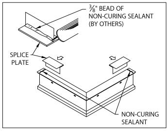
3. ANCHOR BAR MITER SPLICE PLATES APPLY A  $\frac{3}{8}$ " BEAD OF NON-CURING SEALANT (BY OTHERS) TO THE RIGHT ANGLE INTERSECTION OF THE DECK FLANGE AND TO EACH END OF ANCHOR BAR MITER. SLIDE 31/2" WIDE SPLICE PLATE HALFWAY ONTO EACH END OF MITER AS SHOWN.
