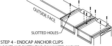
LOCATE AND FASTEN TWO GALVANIZED ANCHOR CLIPS TO THE WALL WITH PROVIDED FASTENERS FOR SUBSTRATE, AS SHOWN IN DETAIL A.
