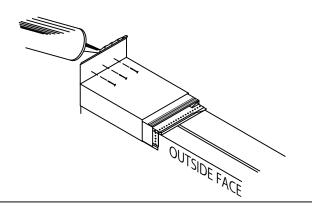
STEP 9 - ENDWALL FLASHING SPLICE PLATE VERSION STEPS 9 - 10 NOTE: WITH THE ENDWALL FLASH SPLICE PLATE VERSION THERE IS ONE ANCHOR CLIP.
