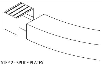
NOTE: ANCHOR CLIPS WIDTH WILL BE DETERMINED BY RADIUS SIZE AND MATERIAL. ALL SPLICE PLATES ARE PROVIDED. REMOVE RELEASE PAPER LEFT TWO SEALANT STRIPS. INSERT SPLICE PLATE HALFWAY INTO THE RIGHT END OF RADIUS SECTION.
