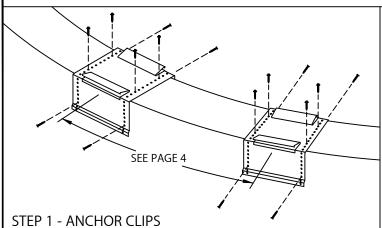
NOTE: RADIUS WILL HAVE DOUBLE SPRING ANCHOR CLIPS. ANCHOR CLIPS WIDTH WILL BE DETERMINED BY RADIUS SIZE AND MATERIAL. LOCATE AND FASTEN ANCHOR CLIPS WITH PROVIDED FASTERNERS FOR SUBSTRATE. SEE PAGE 4, AND ANCHOR CLIP SPACING.
