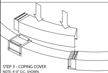
REMOVE RELEASE PAPER FROM RIGHT TWO FACTORY APPLIED SEALANT STRIPS ON THE SPLICE PLATE ON THE COPING SECTION. INSTALL RADIUS COPING SECTIONS FROM LEFT TO RIGHT. PLACE COPING INTO POSITION AND PRESS DOWNWARD UNTIL SNAPLOCK OCCURS.
