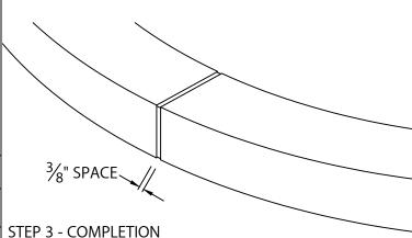
USING RADIUS SECTIONS TO COVER ALL EXPOSED CLIPS / SPLICES, CUT TO LENGTH AS NEEDED USING A FINE TOOTH HACKSAW, SNIPS , OR CUT-OFF WHEEL LEAVING A CLEAN EDGE. BE SURE TO LEAVE A 3/8" SPACE AT EACH JOINT.
