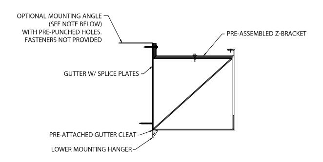
NOTE: IF EXTERIOR OF THE BUILDING CONSISTS OF AN INSULATED PANEL, EIFIS, OR OTHER NON-STRUCTURAL MATERIAL, A MOUNTING ANGLE IS REQUIRED WITH THE LOWER MOUNTING HANGER.
