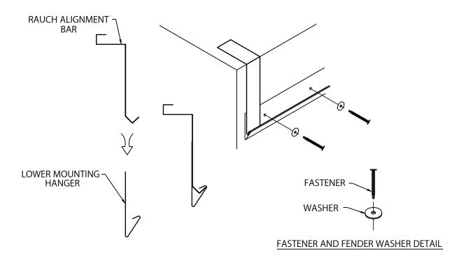
NOTE: RAUCH ALIGNMENT BAR IS NOT PART OF ASSEMBLY. IT IS A TOOL PROVIDED WITH THE GUTTER TO HELP WITH THE ALIGNMENT OF THE INSTALL. THE RAUCH ALIGNMENT BAR HELPS THE CONTRACTOR HOLD THE LOWER MOUNTING HANGER IN PLACE AS IT IS GETTING FASTENED TO THE WALL. THE RAUCH ALIGNMENT BAR IS INTENDED TO RECESS THE GUTTER TOP APPROXIMATELY  $\frac{1}{4}$ " FROM THE TOP OF THE WALL, TO ALLOW FOR WALL VARIATIONS.
