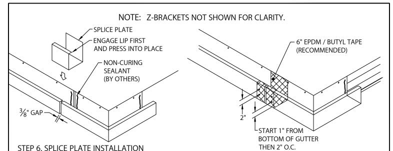
APPLY A HEAVY BEAD OF NON-CURING SEALANT TO INSIDE END OF GUTTER. LEAVE A 3/8" GAP AT SPLICE JOINT. PLACE 6" WIDE SPLICE PLATE AT JOINT. RIVET SECTIONS WITH PROVIDED  $\frac{1}{8}$ " STAINLESS STEEL POP RIVETS AT SPLICE JOINT 2" O.C. AS SHOWN, STARTING 1" FROM BOTTOM OF GUTTER. THE MANUFACTURER RECOMMENDS THE APPLICATION OF EPDM / BUTYL PRESSURE SENSITIVE TAPE CENTERED OVER THE SPLICE PLATE AND LAPPING THE GUTTER SECTIONS A MINIMUM OF 1".
