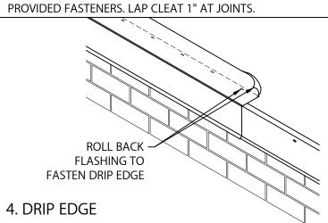
ROLL BACK FLASHING TO EXPOSE FASTENING SLOTS AND FASTEN THRU PRE-SLOTTED HOLES 6" WITH PROVIDED FASTENERS.
