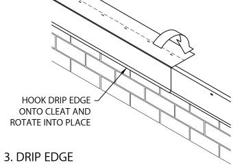
HOOK DRIP EDGE OF EACH DRIP EDGE SECTION ONTO CONTINUOUS CLEAT, ROTATE INTO PLACE.
