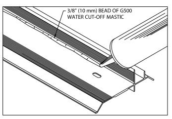
2. Miter & Scupper Anchor Bar (Preparation) Lay miters and spillout scuppers on deck with outside face down. Be sure aluminum anchor bar is clean and free of dirt or dust. Apply a heavy 3/8" (10 mm) bead of G500 Water Cut-Off Mastic to the right angle intersection of the deck flange and back of anchor bar as shown. Application of sealant is required along the full length of each miter anchor bar.
