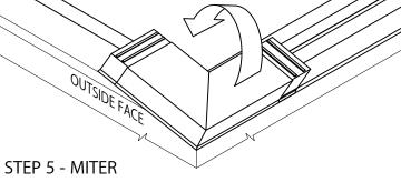
HOOK OUTSIDE FACE OF MITER ASSEMBLY ONTO CONTINUOUS CLEAT AND ROTATE INTO PLACE.
