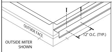
STEP 3 - CONTINUOUS CLEATS AT CORNERS FASTEN ONE OUTSIDE CONTINUOUS CLEAT 12" O.C. WITH PROVIDED FASTENERS (SEE DETAIL A).
