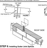
Locate the joint splice for the appropriate gutter. Apply a continuous bead of non-curing sealant to both sides of the joint. Slide the joint splice down into the gutter. Secure the joint splice in place by pop riveting it on the high side of the joint (FIGURE 1) on the 3 surfaces as shown in FIGURE 2. There must be a joint splice at every joint.
