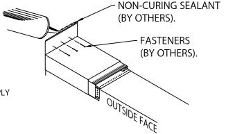
STEP 9 - ENDWALL FLASHING SPLICE PLATE VERSION STEPS 9 - 10 NOTE: WITH THE ENDWALL FLASH SPLICE PLATE VERSION THERE IS ONE ANCHOR CLIP.
