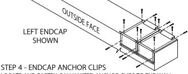
LOCATE AND FASTEN GALVANIZED ANCHOR CLIPS TO THE WALL WITH PROVIDED FASTENERS FOR SUBSTRATE, AS SHOWN IN DETAIL A. FOR FASTENER DETAIL SEE PAGE 4.
