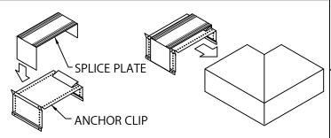
STEP 2 - MITER SPLICE PLATES & ANCHOR CLIPS REMOVE RELEASE PAPER FROM SPLICE PLATE SEALANT STRIPS. POSITION THE SPLICE PLATE IN THE CENTER OF THE ANCHOR CLIP. INSTALL THE SPLICE PLATE AND ANCHOR CLIP ASSEMBLIES HALFWAY INTO EACH END OF THE CORNER MITER AS SHOWN.
